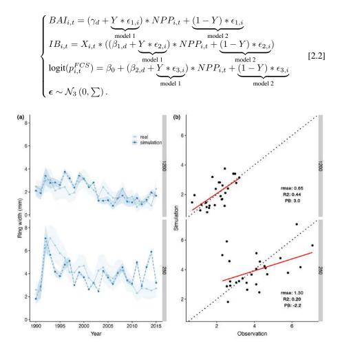
**Figure 2.4.** Comparison of observed and simulated ring width from 1989 to 2015 and for two stand densities. a) Observed data are shown in light blue, while simulated ring widths are shown in dark blue. Mean values are shown along with standard deviations (broader strip). b) The dashed black line corresponds to the 1:1 line, and the red line corresponds to the regression between simulated and observed ring width values. For a color version of this figure, see www.iste.co.uk/peyrard/ecology.zip
